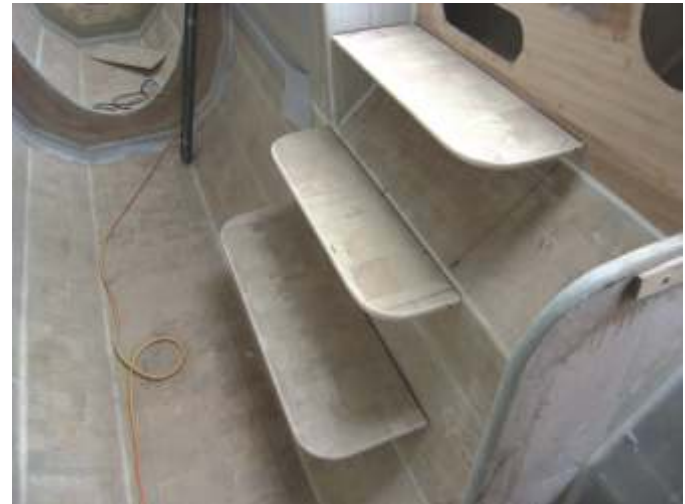
Little things like good stairs into the hulls. Very fetley to do but if they are wrong they will be a nuisance every day you liveaboard. The ones below give access forward and steps up to our cabin. Another dent in the scrap supply..
