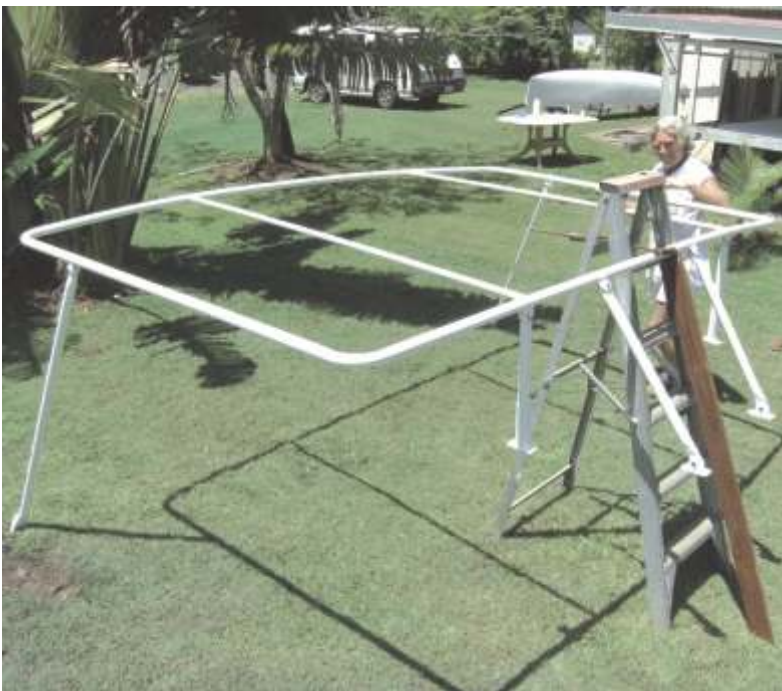
Another problem soon to face is a cockpit canopy. We like the idea of visual access over the top of the main cabin so the extension type won't do for us. Neighbour Malcolm Salisbury is working on one for his Crowther Catana, Coconut Airlines , and though we may want ours lower, the aluminium frame and Polycore top may be a good solution for our boat. So we'll keep an eye on his progress as well as another boat in the harbour, Giddy-up go who is doing something similar. If theirs works out well, we will shamelessly steal the plans!
