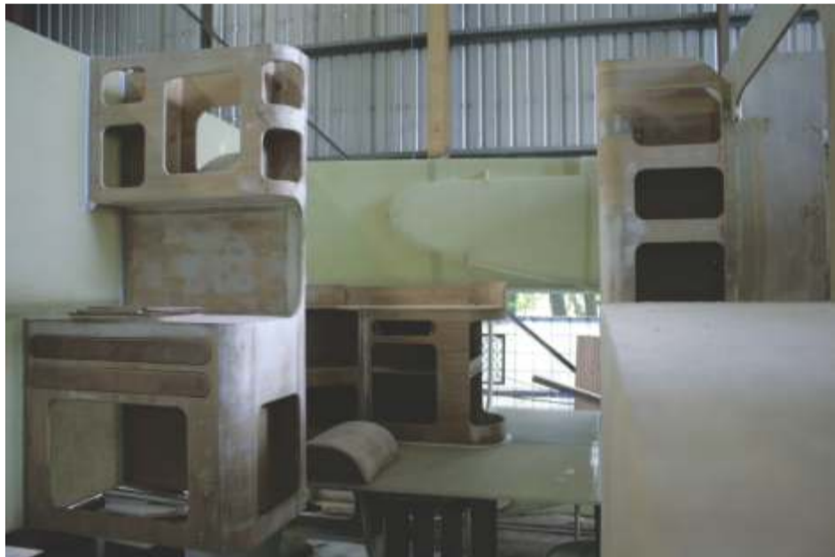
Ian chose Kauri for fitout timber but regrets it as the wood wasn't stable. It would lose its shape overnight after installation and require more work to straighten out.
